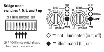
Mode switch settings and LED indication for parallel mode operation. BRDG indicator and PAR indicator should be illuminated when in bridge mode.
